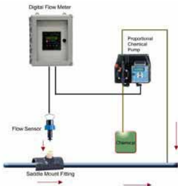
Typical injection system treats water proportional to flow in the main water line.
